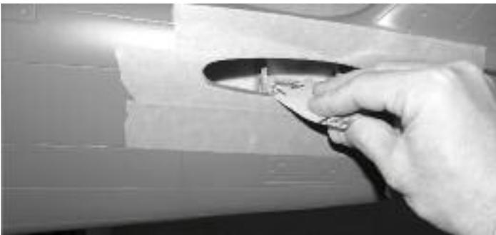
41. To make epoxy cleanup easier, apply masking tape to the fuselage and stab as shown. Sand the elevator saddle with 100 grit sandpaper to remove the existing paint and primer. This will help the elevator bond to the fuselage.
