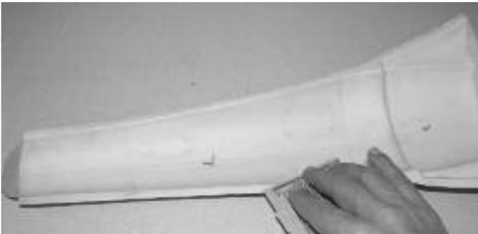
35. Sand the edges of the belly pan with 100 grit sandpaper to remove any mold release or high spots and clean with rubbing or denatured alcohol. Also clean the wing with denatured alcohol in the area that was marked in the previous steps.
