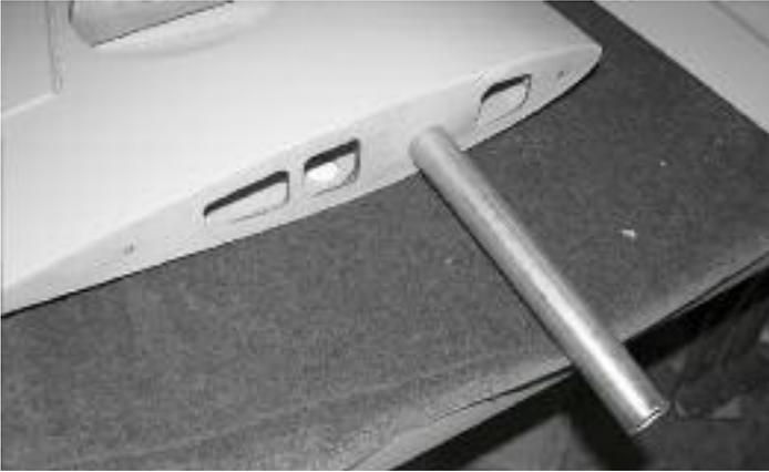
17. Fit the aluminum tube in the wings and assemble the wing halves to check for a good fit. Sand or adjust the root ribs as necessary so there are no gaps.
