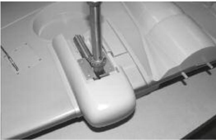
103. Correctly fit the fiberglass gear covers in place and mark their location on both sides of the wing. Small variations in the wing frame up may cause the gear pods to not fit exactly. You can use a heat gun to make small adjustments or cut the inside of the gear pods, along the gear mounts so they fit the wing correctly.
