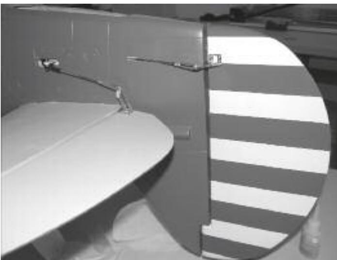
89. Measure and cut the rod to length using the same method as the elevator. Note: The servo arm will point towards the center of the fuselage and the pushrod will exit the fuselage on the opposite side as the servo. (see tail wheel retract photo)
