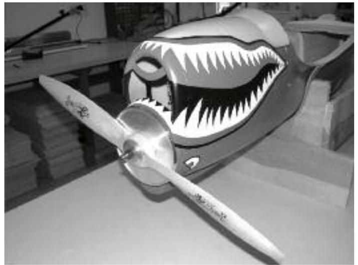
57. Attach the spinner backplate and prop to the engine and align the backplate with the front of the cowl. There should be a 1/8" gap between the spinner backplate and the front of the cowl. Note: You will be able to move the engine box slightly to center the engine. If you can't adjust the engine box as much as is required, then you may need to make a small adjustment of the cowl in order to fit it perfectly to the spinner backplate.
