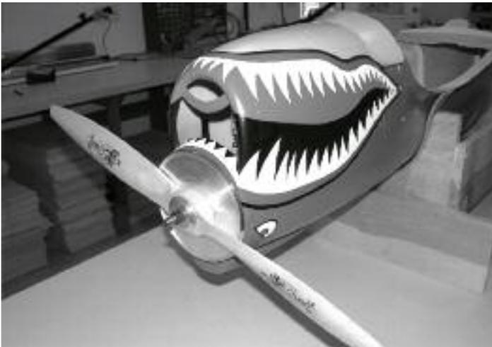
64. Re-fit the engine box in the fuselage and attach the cowl with the provided #2 x 3/8" button head screws and plastic washers.
