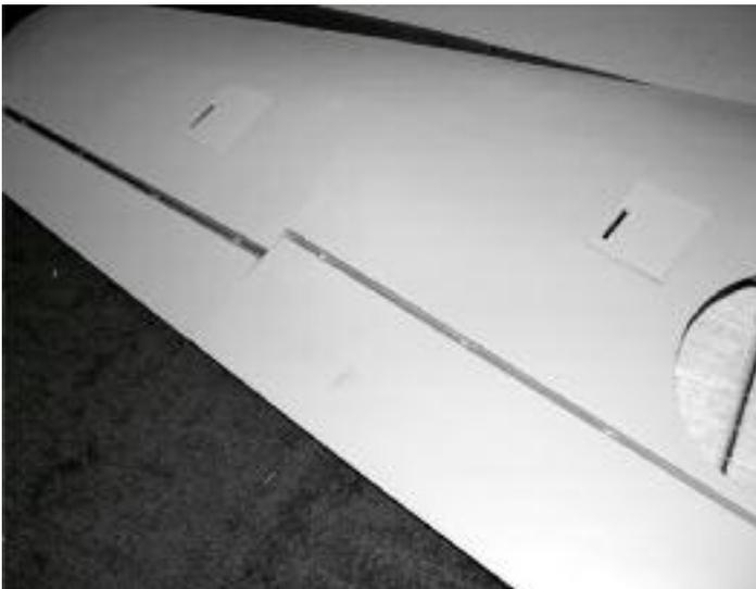
3. Test fit the servo covers in the wing holes. The slots in the wing covers should be positioned as shown in the photo. This will insure that the pushrods line up with the hardwood blocks in the ailerons and flaps.
