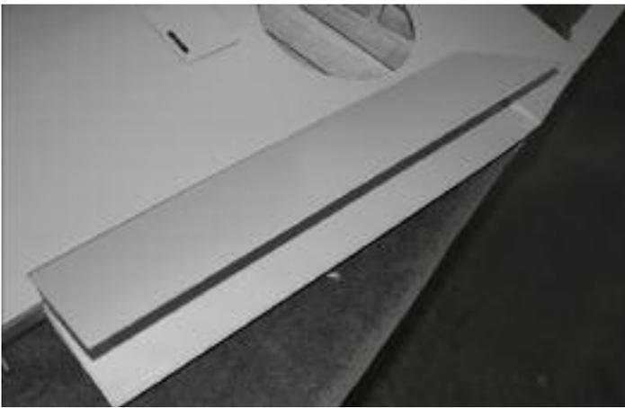
6. Insert the hinges into the flap and trailing edge of the wing. Check for proper alignment and operation of the flap. Realign the hinges as necessary. Note: The hinges will be inset into the flap leading edge so the gap will be minimized.
