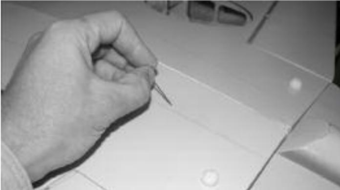
34. Remove the belly pan and use a pin to poke holes in the covering along the inside of the lines you just made.
