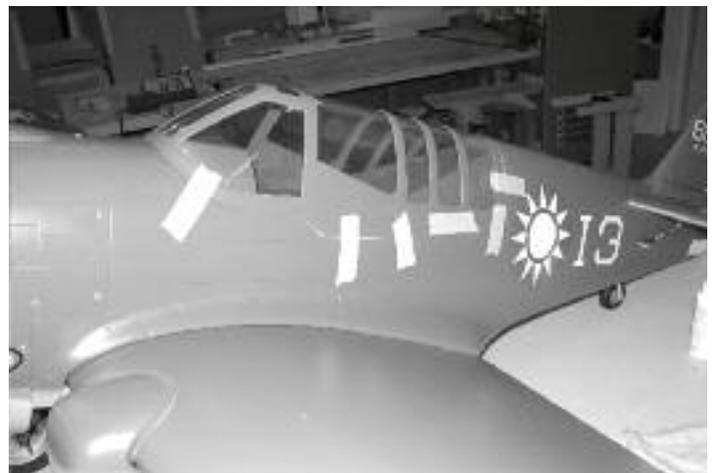
112. Carefully cut the canopy along the formed lines and test fit on the fuselage.
