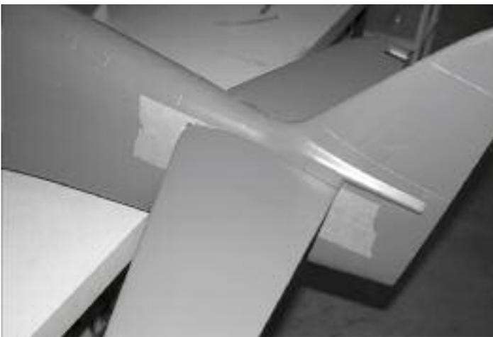
42. Apply a 1/2" wide strip of 5 or 30 min epoxy to the inside of the line you made on each side of the horizontal stab.
