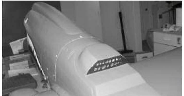
110. Use 5 min epoxy to glue the instrument panel to the cockpit.
