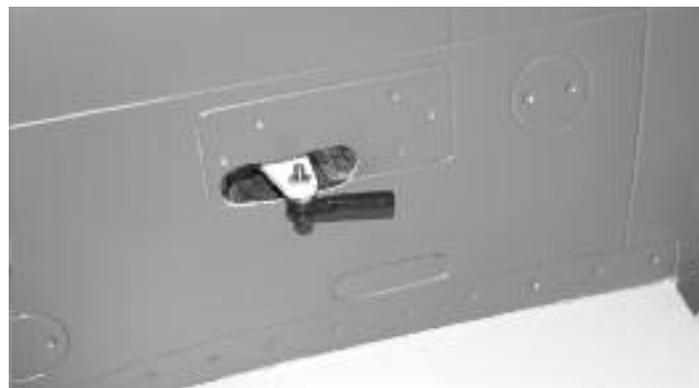
72. Connect the 4-40 ball link adapter to the control arm and install the arm on the servo.
