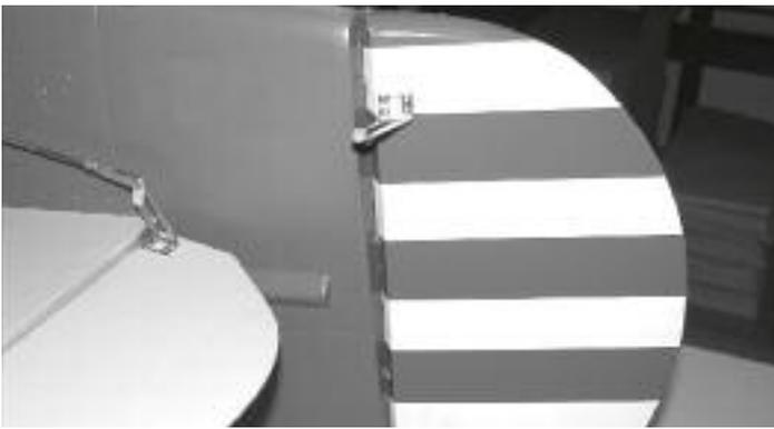
85. Measure 1-5/8" up from the bottom of the rudder and install a 1-1/8" control horn using the same method as the elevator horns.
