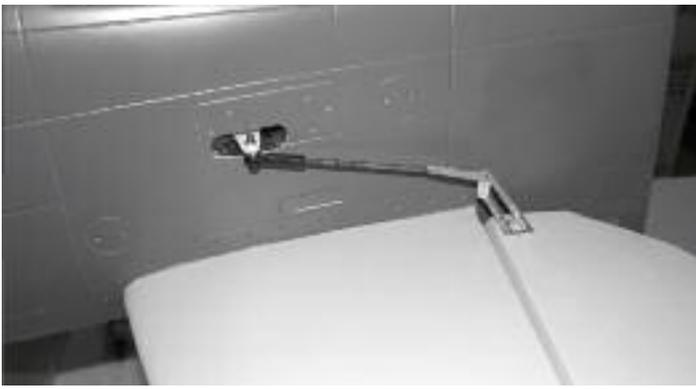
77. Re-install the control arms on the servos and connect the clevises to the control horns. Adjust the length as necessary by threading the rod in or out of the plastic swivel link arm or clevis. Tighten the lock nuts and use thread locking compound to secure them in place.
