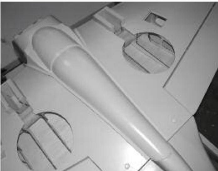
31. Bolt the wing to the fuselage and test fit the belly pan to the center of the wing bottom
