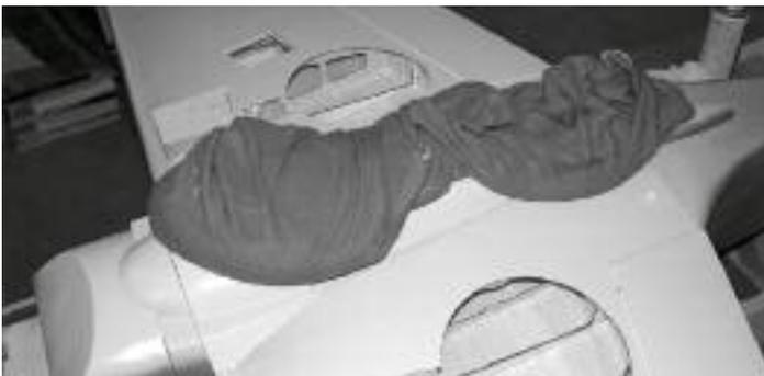
36. Apply 5 or 30 minute epoxy to each mounting edge and fit the belly pan to the wing. Apply weight to the belly pan until the epoxy has cured. We use socks filled with lead shot for this task but magazines or plastic bags filled with sand also work.
