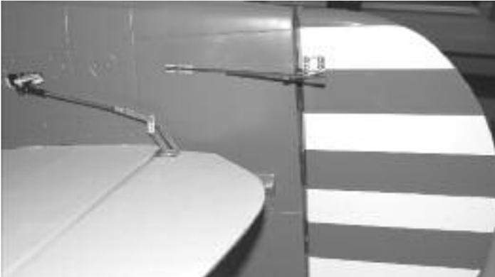
86. Install a high torque metal gear servo in the rear fuselage tray on the opposite side as the rudder control horn.
