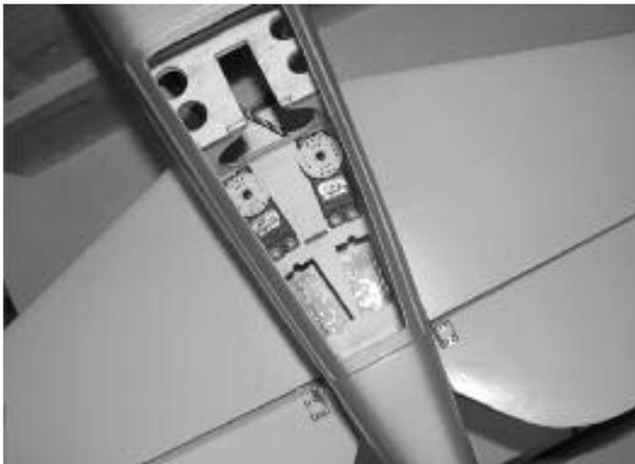
69. Install two high torque servos in the forward most slots on the rear fuselage servo tray as shown. Note: You will need long control arms for these servos.
