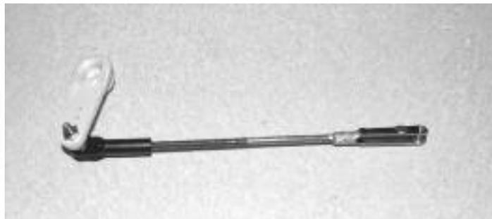
75. Remove the control arm/rod/clevis assembly and make another rod the same length for the other elevator half. Assemble both pushrods with a ball link adapter and 4-40 lock nut on one end and 4-40 clevis and lock nut on the other end.
