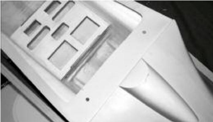
30. Enlarge the fuselage wing mounting plate holes to 19/64" and install the 1/4-20 metal blind nuts securely on the back side using CA or epoxy. Note: Do not use the nylon 1/4-20 bolts to set the blind nuts in the plywood because they are not strong enough. The best way is to use a spare 1/4-20 metal bolt or strong pliers.
