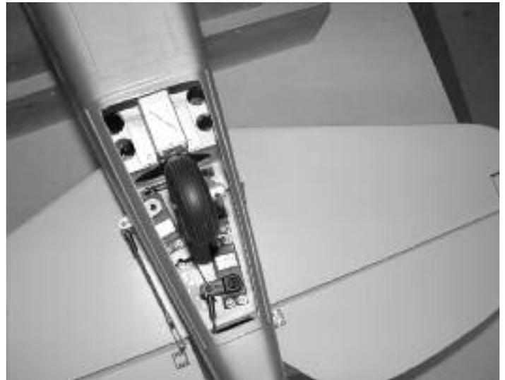
91. Align the tailwheel retract as shown. It should sit back at least 3/16" from the rear edge of the plywood mounting plate. Add a 2" tail wheel and check for servo clearance. Adjust the position as necessary for proper clearance.
