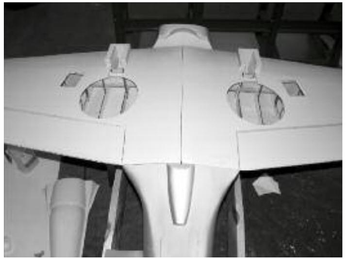
26. Place the wing on the fuselage and double check the wing dowel alignment. Once everything is aligned, drill two 1/4" holes in the fuselage wing dowel plate at the marked locations.
