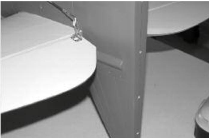
80. Mark and drill three evenly spaced 1/8" hinge holes in the vertical stab.
