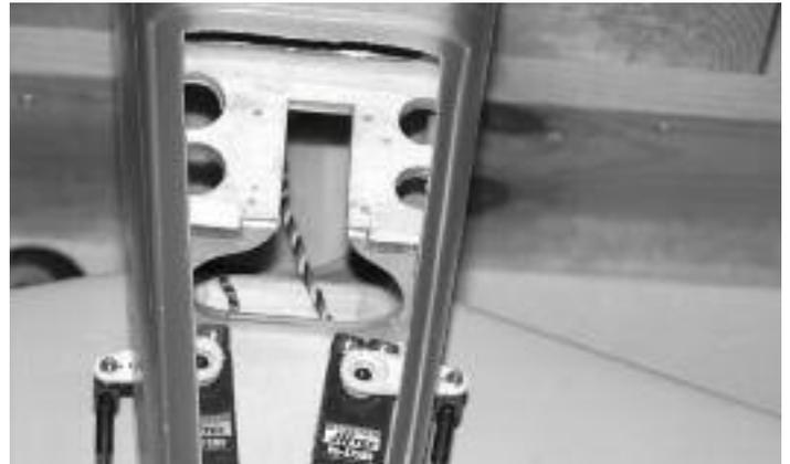
92. Mark and drill four 3/32" mounting holes. Remove the retract and put a few drops of thin CA in each hole.
