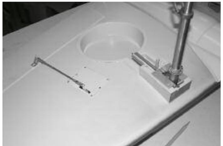
100. Mark a line around the wheel well covers and remove the covering in that area.
