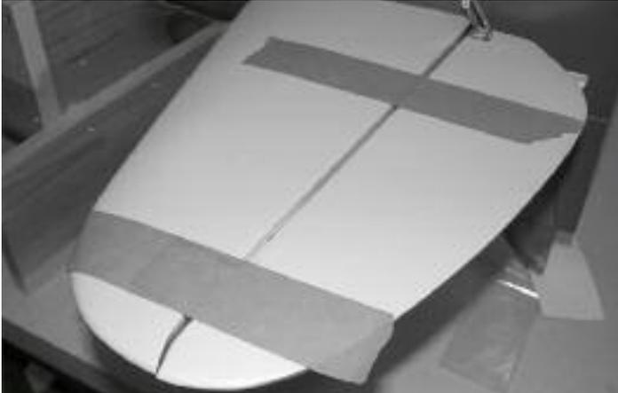
47. Hinge the elevators to the H stab using the same method as was used with the ailerons. Tape in place and allow the epoxy to cure.
