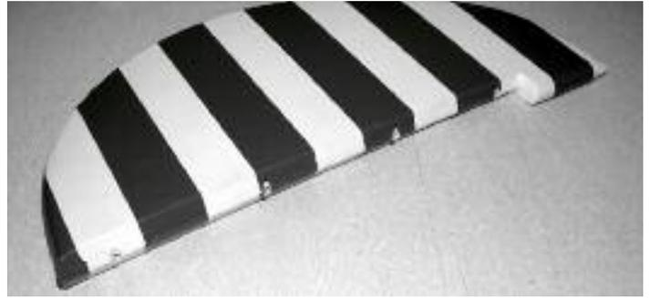
81. Mark the the holes in the same location on the rudder and drill to 1/8". Note: You may want to cut a small slot in the beveled edge of the rudder at each hinge location to make drilling easier.
