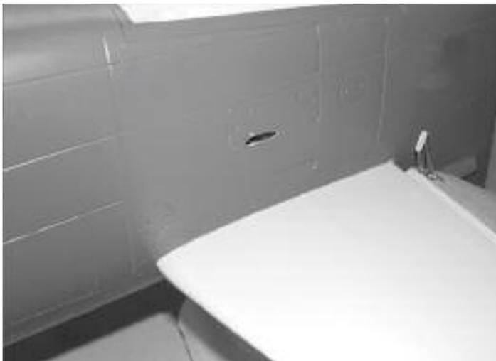
70. Note the location of the servo arm on the inside of the fuselage. Mark the location on the outside of the fuselage.
