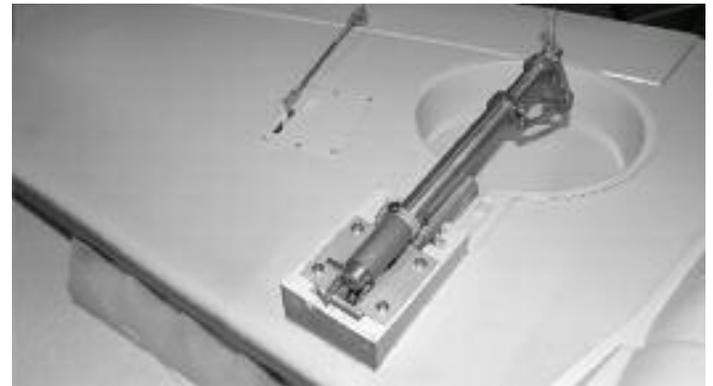
99. Carefully cut the abs wheel well covers along the scribed lines and fit in place as shown. You will also need to drill holes in the cover so the airlines on the end of the cylinder can be routed into the wing. Note: You may need to cut slots in the ribs so you have room to fit the servo wires with the wheel well cover in place.
