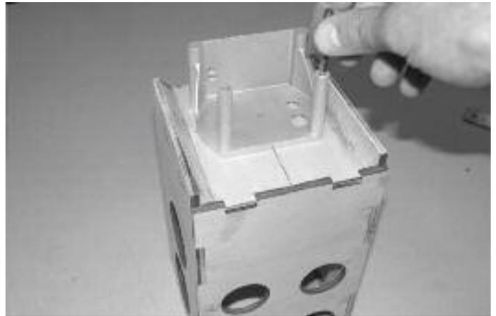
50. Center the engine mount on the firewall box with the marks made in the previous step.
