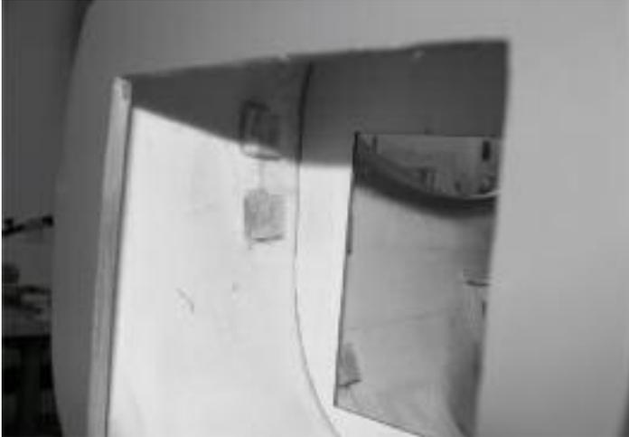
62. Use 5 min epoxy to attach a hardwood block to each hole location inside the fuselage. These will act as the screw backup when you attach the cowl. The reason you do this now is because after the firewall box is in place, you won't have access to this area - so make sure they are glued in place well!
