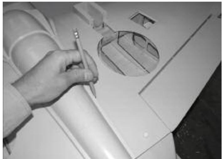
33. Once you have a good fit, remove the tape on one side of the belly pan and mark a line on the wing at the edge of the belly pan. Repeat for the other side.
