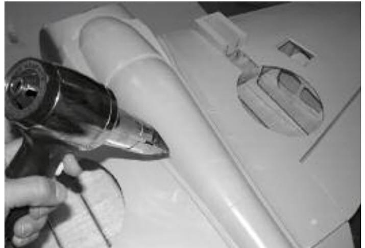
32. If your belly pan doesn't fit exactly (turned up edges, wrong contour, etc) you can adjust it by taping the edges with masking tape and using a heat gun to soften the fiberglass while carefully pressing it into place with a gloved hand. You may need to go over it a couple times, letting it cool in between. Note: Be careful not to bend the fiberglass too much while it is cool or the paint will crack.
