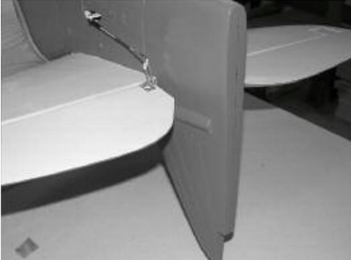
79. Measure and draw a line down the center of the vertical stab as shown.
