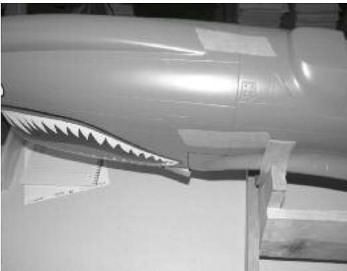
56. Slide the firewall box into the fuselage and tape the cowl in place along the molded lines on the fuselage
