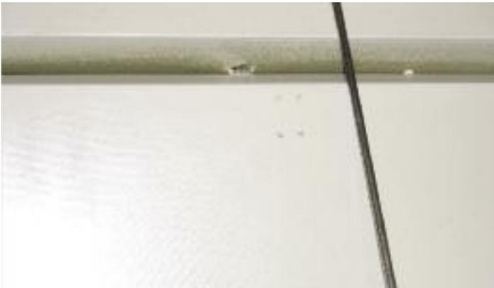
12. Mark the location of the control horn. Remove the horn and drill four 3/32" holes at the marked locations. Use the enclosed 2-56 x 1.5" screws to attach the control horn to the elevator and backplate.
