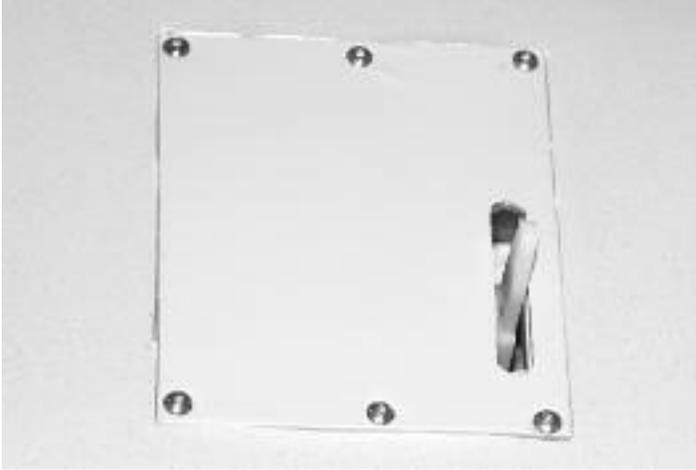
10. Use a 1/16" drill bit to drill holes in the servo hatch and mounting plate as shown. Make sure to drill close enough to the edge of the hatch so you also drill into the mounting blocks below. Secure the hatch using (6) #2 x 3/8" button head screws.
