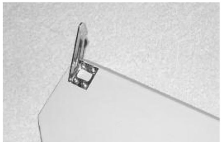
46. Attach the control horn to the backplate using four 2-56 x 1-1/2" screws. Repeat for the other elevator half. Note: Make sure the control horns are in the same location on each elevator half.
