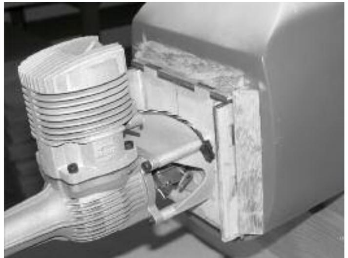
67. Remove the spinner, prop and cowl and use the hardwood tri-stock and 5 min epoxy to secure the firewall in place. Place the tri-stock as shown. Note: you can also sand the front of the firewall where the tri-stock fits for better adhesion of the epoxy.
