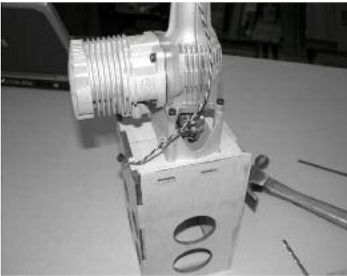
54. Install the motor and mount onto the firewall. Note: you may need to drill out the mount bolt holes to 15/16" because sometimes the blind nuts will extend through the firewall a little. Either that, or you can epoxy a piece of 1/8" ply to the back of the firewall before installing the blind nuts. This will increase the thickness of the firewall so the blind nuts don't extend all the way through.
