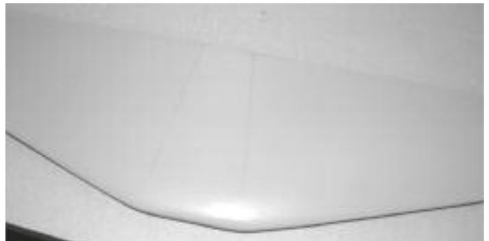
39. Draw a line on each side of the stab where it meets the fuselage. Do this on the top and bottom of the stab.
