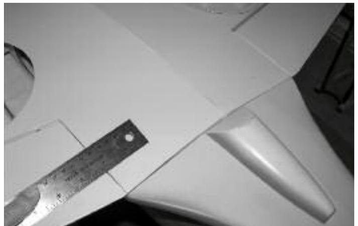
28. With the wing centered, measure 2-1/2" over from the flap and 1" up from the wing trailing edge. Make a mark in this location on each wing half.
