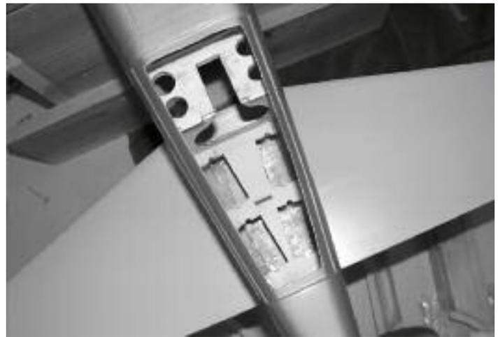
44. When the epoxy cures completely, remove the masking tape and inspect the stab to insure it is well glued. If there are any missed spots, apply epoxy to fill the gap. You can clean up any additional epoxy with denatured alcohol. Note. You can access the bottom of the stab through the tail wheel retract area. Apply a thin layer of epoxy to the stab in this area in insure everything is secure.
