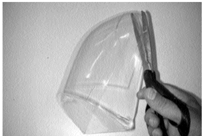
153. Carefully cut the canopy along the formed lines.
