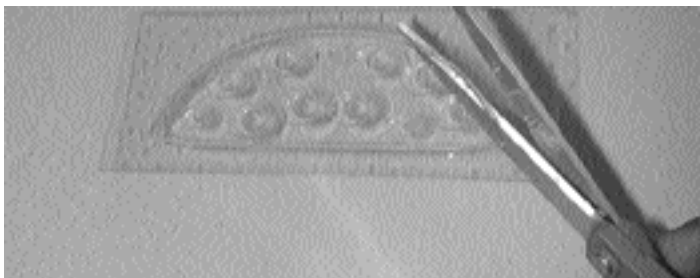
146. Cut the clear plastic lens cover piece around the outside line.
