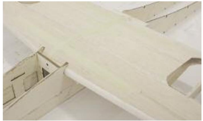
15. At the back of B2, score the balsa sides about half way through on the inside. This will allow you to bend the fuselage easier.
