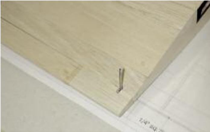
51. Glue two 1" tapered trailing edge pieces to the outboard end of the wing trailing edge with medium CA.
