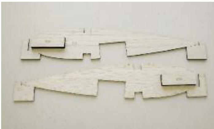
18. Locate two R1 ribs and glue on R1A balsa wing dowel block on the outboard side of each R1 rib as shown on the plan. Make sure you have a right and left.
