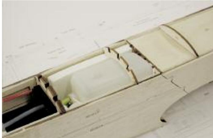
44. Align B4 with the scribed line on C1 and sand the bottom of B4 so it will match the angle shown on the plan [8L]. Glue B4 to C1 aligning it with the scribed line. Test fit B5 4" back from F1 and glue in place. *You may need to cut part of B5 so the fuel tank will fit.* Align and glue the B6 assembly on top of F1.
