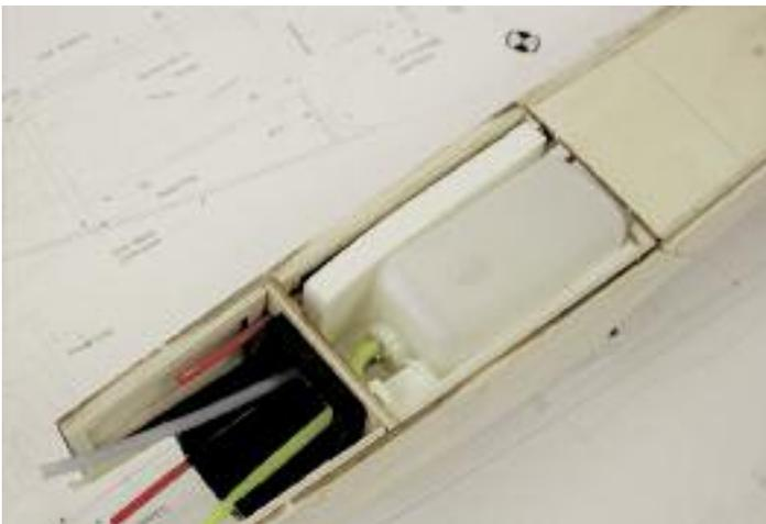
42. Now you are ready to install the fuel tank. Assemble fuel tank and set tank into the tank compartment. Determine necessary foam padding to hold tank in the center so that it will be even with the engine carburetor. Run fuel lines through the firewall.
