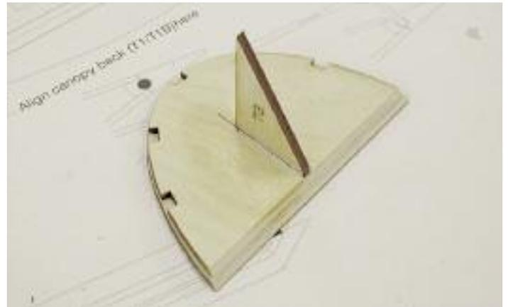
35. Bevel bottom of 1A/1B assembly. Center and glue TG backrest flush with bottom.
