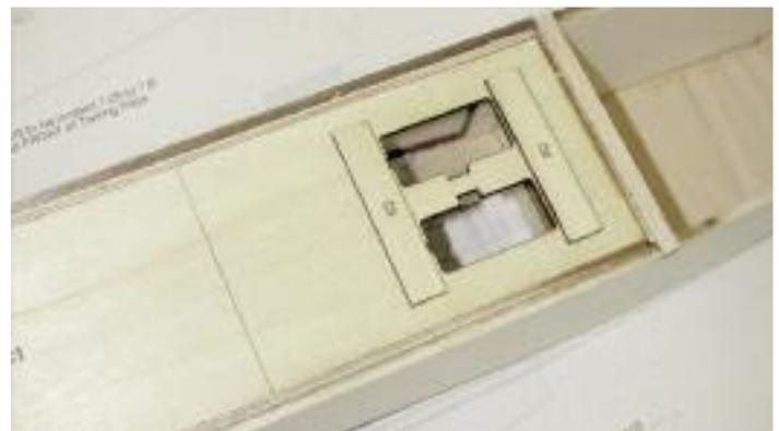
33. Run the flexible control rods from the holes in the rear of the fuselage to the holes in B2. Glue in place with medium CA.
