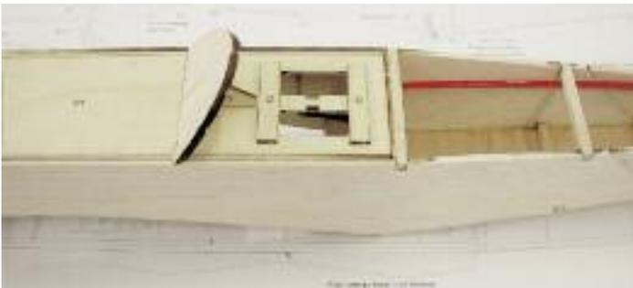
36. Align the front of TG to the scribed line in C2. Adjust the length of TG to fit around C3. Glue in place with medium CA.
