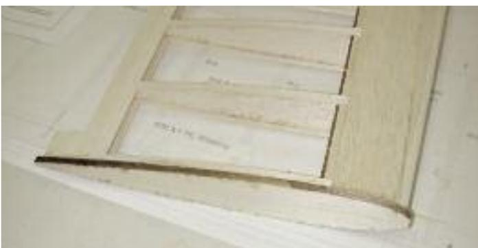
54. Align and glue WT wingtip blocks in place flat against R11 using medium CA.
