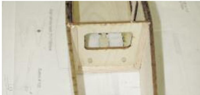
20. Cut and fit 1/4" sq. vertical pieces and glue to B2 and fuselage sides.
