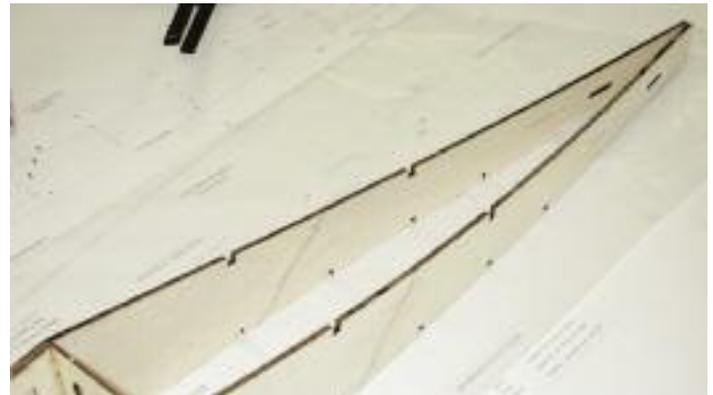
17. Locate and glue with 5 min epoxy PW so that it fits flush with the top of the cut-out for the horizontal stab. This can be done while the fuselage is pinned to the building surface or you can unpin the fuselage and turn it over as show in the photo.
