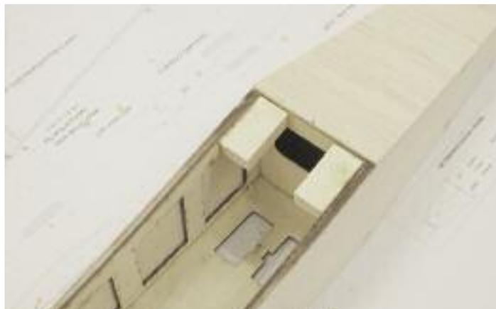
23. Locate the two 7/8" x 1/2" x 1-5/8" wing hold down blocks. Bevel each block so it will fit flush with B2 and parallel with wing saddle.
