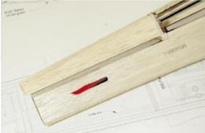
55. Once the blocks are sanded to shape, remove and discard the spacer. The blocks should now have a taper that matches the stringer angle as shown in photo. Sand the rear of the blocks to match the fuselage length.
