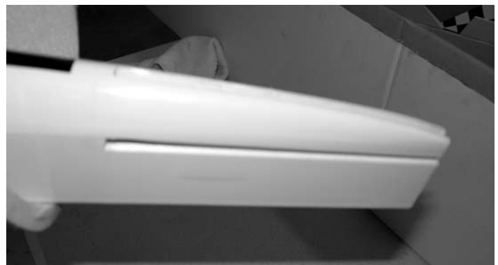
36. Use a sharp hobby knife or hot soldering iron to remove the covering from the horizontal and vertical stab slots in the rear of the fuselage.
