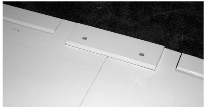
33. Turn the wing upside down and test fit the wing bolt mounting plate. Once it is positioned properly, use a pencil to mark a line around the plate.
