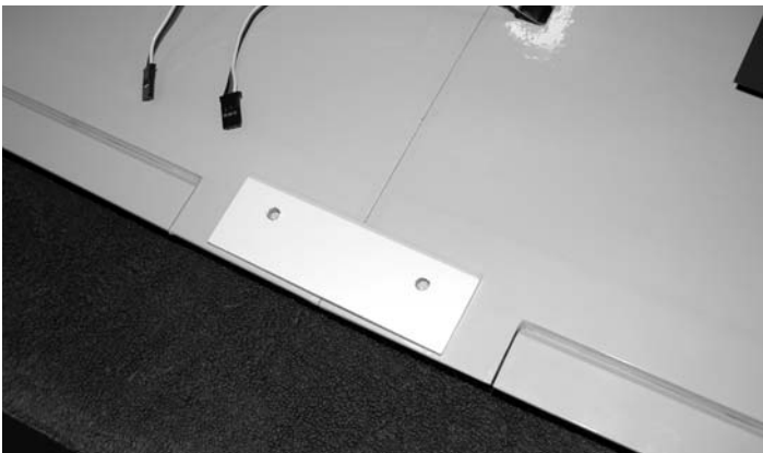
31. Remove the covering from the holes in the plywood wing bolt mounting place and align the plate with the top of the wing so the bolt marks align with the holes in the mounting plate. You may need to adjust the marked holes slightly so they match the holes in the plate
