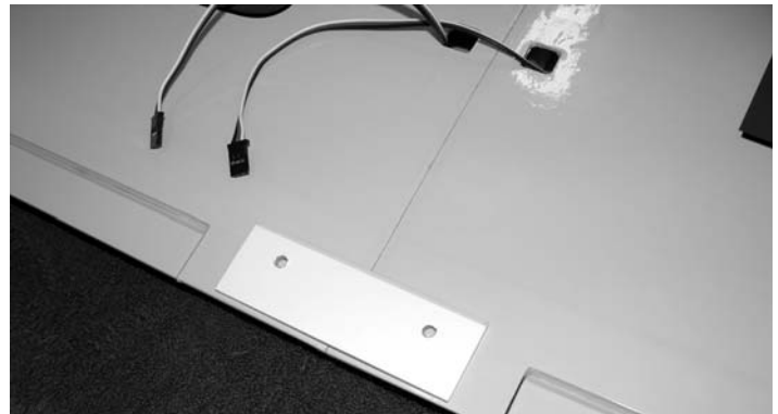
34. Remove the covering 1/18" inside the line you drew being careful not to cut into the sheeting on the wing.
