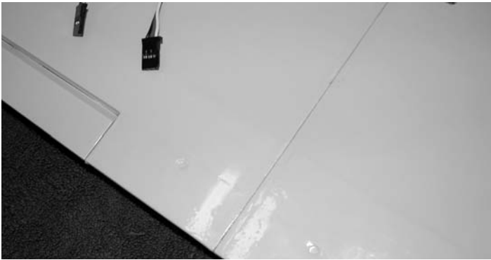
30. Remove the wing from the saddle and use a pencil to make the bolt indentations more visible.
